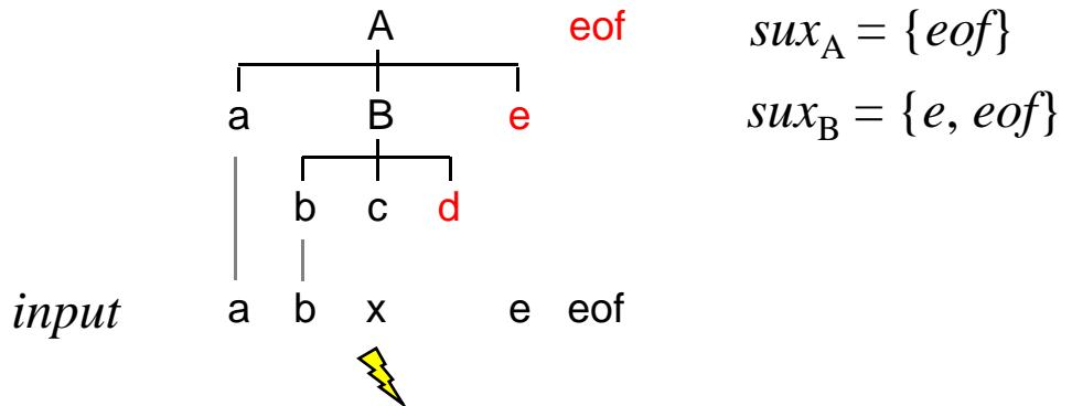
the error is detected here; anchors = {d, e, eof}
