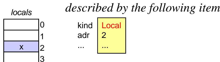
After loading the value with *ldloc.2* it is on *estack*
