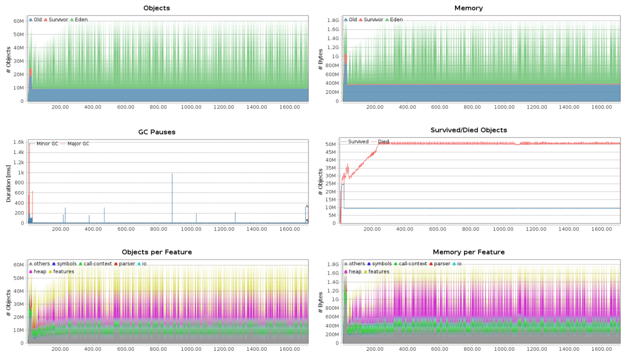
Figure 79: Memory behavior of the AntTracks analysis tool parsing through the memory leaking tradesoap benchmark
