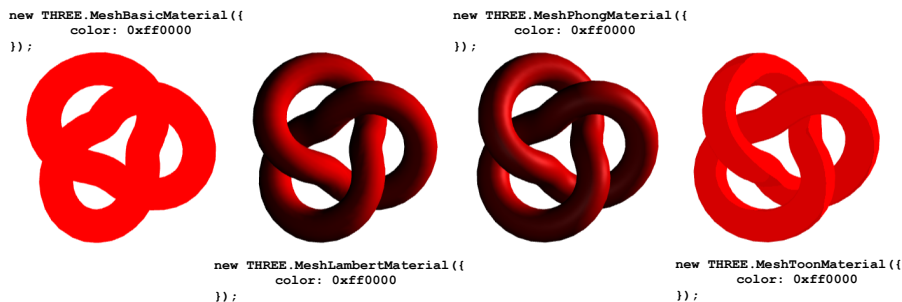
Fig. 17. Materials define how items appear in the scene. More complex and realistic materials work with extra properties such as shininess and roughness.
