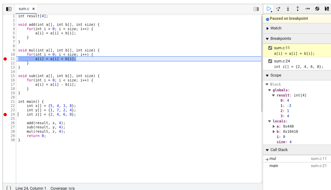
Figure 5.1: DevTools of the Microsoft Edge browser showing the debugging state of a small application.
